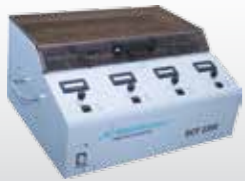
SCF 2300 Flexion test system
